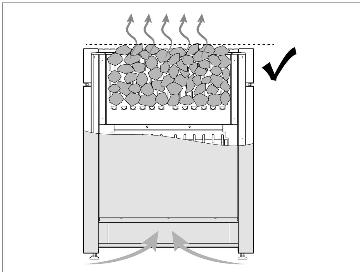
Figure 1. Piling of the sauna stones
