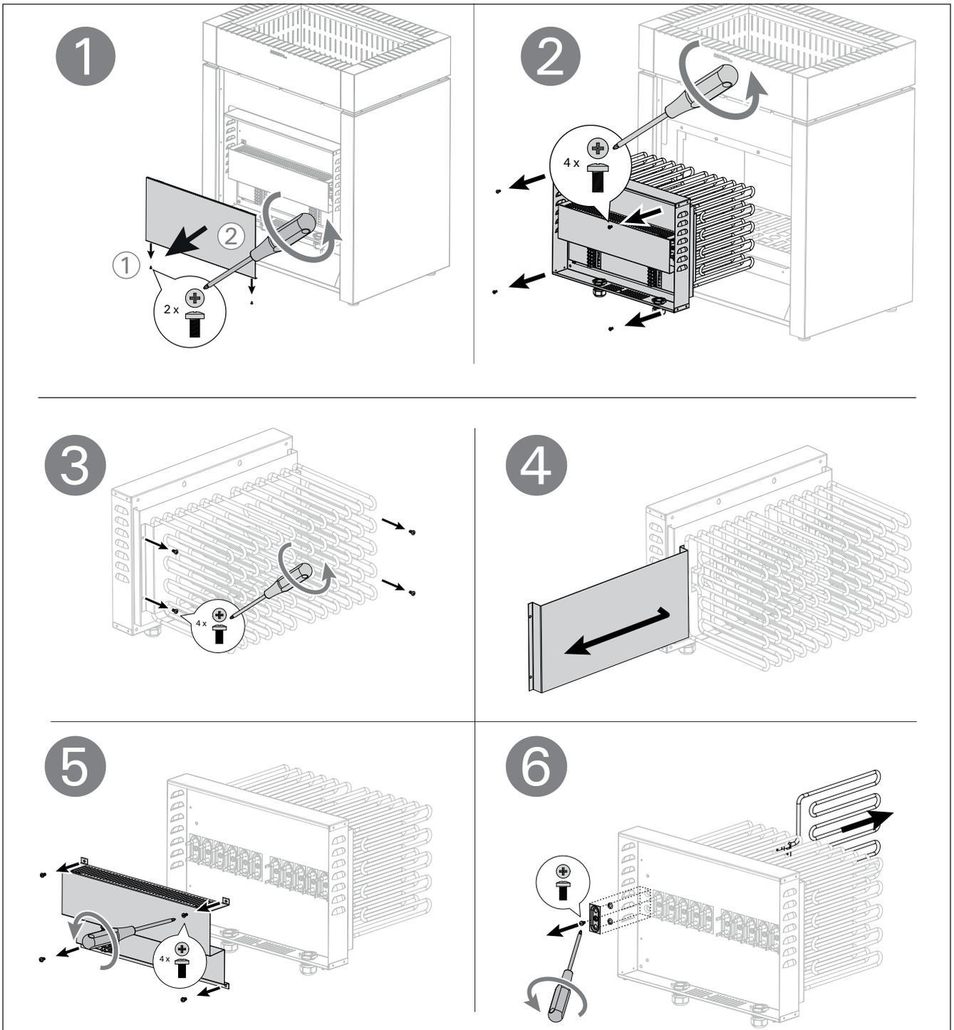
Figure 6. Replacing the Heating Elements
