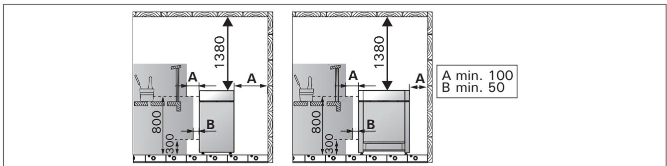
Figure 4. Minimum safety distances (all dimensions in millimeters)
