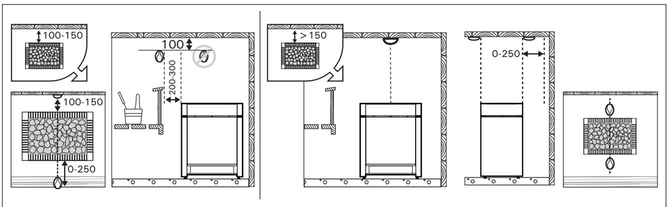
Figure 7. Installing the sensor (all dimensions in millimeters)
