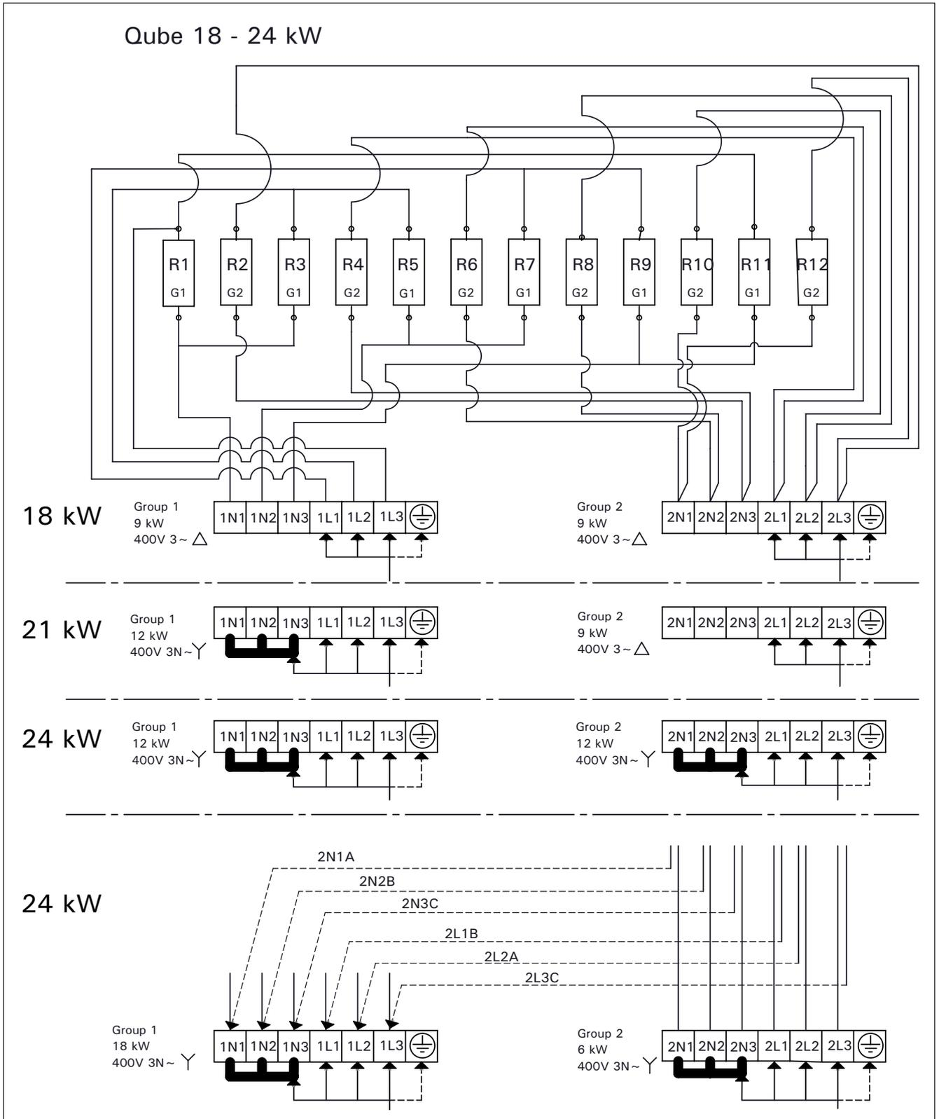
**Figure 8. Electrical connections**
